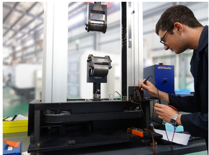
An ADMET engineer performs a diagnostic check on an older universal testing machine
