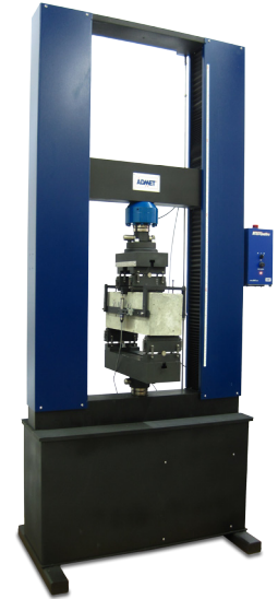
eXpert 2654 100 kN system configured for ASTM C1609 testing
