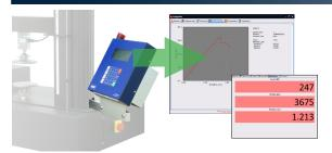
GaugeSafe software is a PC-based data exchange program that communicates with your ADMET controller or indicator via a USB flash (thumb) drive or directly through a USB cable. GaugeSafe software is compatible with the PI-XS, DFG, GaugeBuster 2 and the ep2 indicators as well as the ep2 controller.
