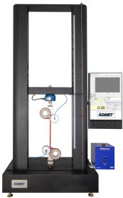
eXpert 2610 - 5kN Dual Column UTM Table top machine equipped with pneumatic rope grips and frame mounted touch panel computer.
