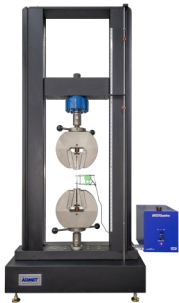
eXpert 2614 - 100kN Dual Column UTM Table top machine equipped with moving body wedge grips and extensometer.
