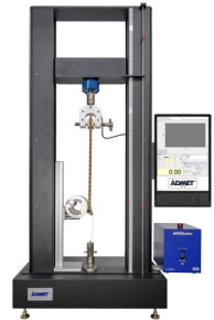
eXpert 2613 - 50kN Dual Column UTM Table top machine equipped with floating roller peel fixture and frame mounted touch panel computer.
