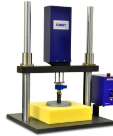
eXpert 5603AF - 1kN Dual Column UTM Table top machine capable of 420 in/min travel for performing B1 IFD and I3 Constant Force Pound tests according to ASTM D3574.
