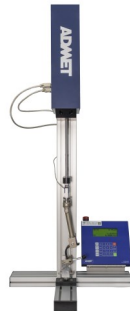
eXpert 5601 - 1kN Single Column UTM Table top machine equipped with custom tension fixture and the standalone eP2 Digital Controller.
