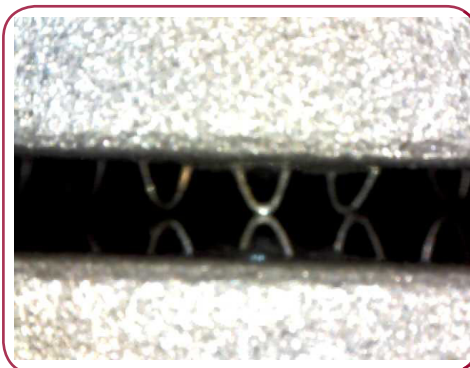
A USB microscope was incorporated to record weld breaks to ensure the tests were run properly.
