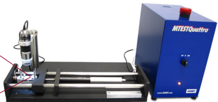
eXpert 4000 series 45N horizontal MicroTester equipped with ADMET's MTESTQuattro(R) controller and 200x microscope for testing the strength of individual stent welds. A custom grip assembly was engineered to quickly load each test sample, isolate a weld and clamp the surrounding wire.
