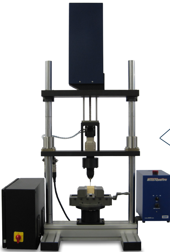
eXpert 8602 (2.2kN/20Nm) Axial Torsion Test System for performing ASTM F543: Test Methods for Determining the Mechanical Properties of Metallic Medical Bone Screws
