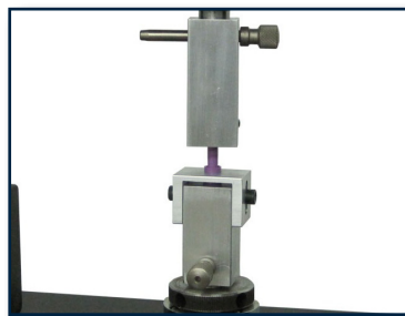
Axial Torsion Test System performing ISO 594 Conical Luer fitting tests
